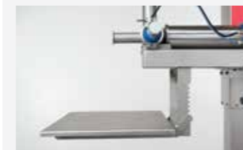
C The working table is manually adjustable (per 5 mm.)
